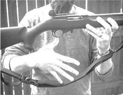
1 Adjust sling so the distance between the bottom of the trigger guard and the sling is equal to one hand width.
